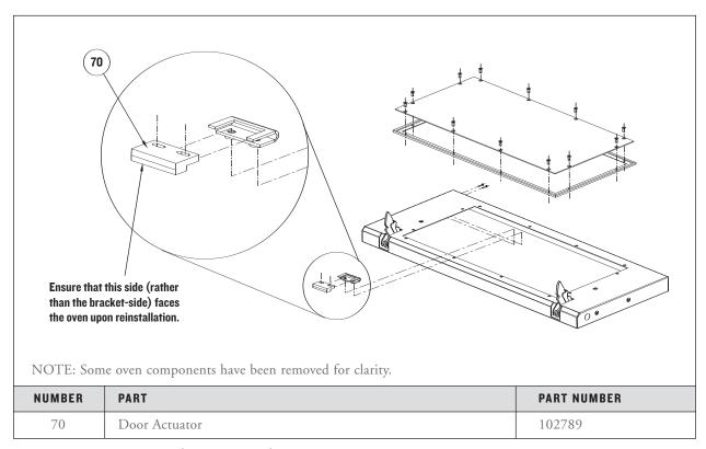
FIGURE 54: Door Actuator and Mounting Bracket
